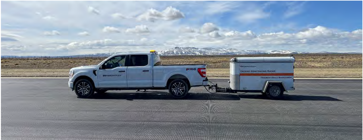
Figure 2-10: The Shannon & Wilson GPR Trailer
