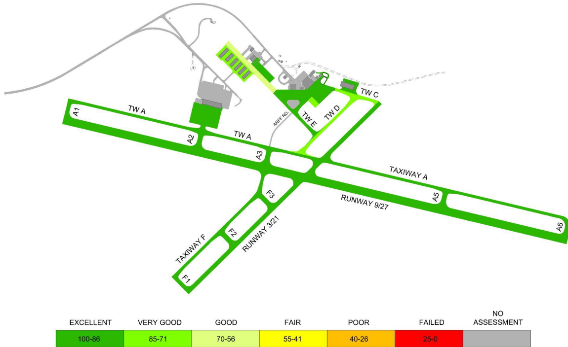
Figure 1.5 Airfield Pavement Conditions (2020)
